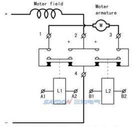
Paired Single Pole Double Throw Contactor for motor reversing 1.2.3.4 Contact Terminal
