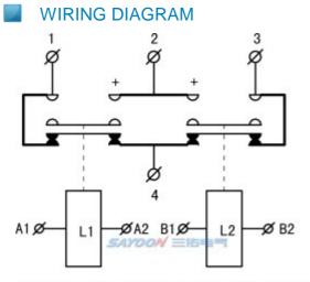
Paired Single Pole Double Throw Contactor. 1.2.3.4 Contact Terminal A1. A2.B1. B2 for the two sets of coil terminal
