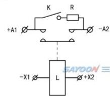
Single Pole Single Throv + Contactor. (One Normal Open) +A1.-A2 Main Contact Terminal
