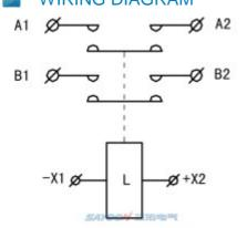
AD Double Pole Double Throw Contactor. (Two Normally Open) A1.A2.B1.B2 Contact Terminal -X1.+X2 Coil Terminal
