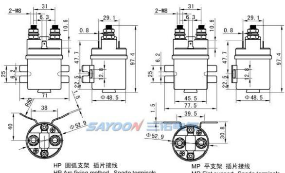
HP Arc fixing method, Spade terminals
