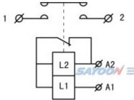
Single Pole Single Throw Contactor. (One Normally Open) 1.2 Contact Terminal A1.A2 Coil Terminal L1 Take-off the winding L2 keep the winding
